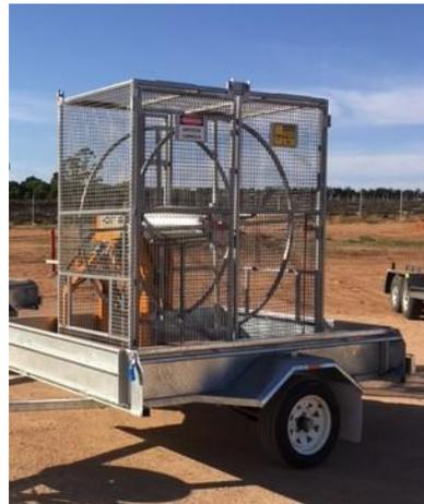
**Photo 2 - A Netafim Recoiling Machine.** Sustaining Endeavour, Netafim and the SA Government have previously assisted three SA regional stores to purchase a machine and trailer to facilitate efficient recycling: McLaren Vale Irrigation, Daish Irrigation (Langhorne Creek) and Graetz Irrigation (Barossa)
