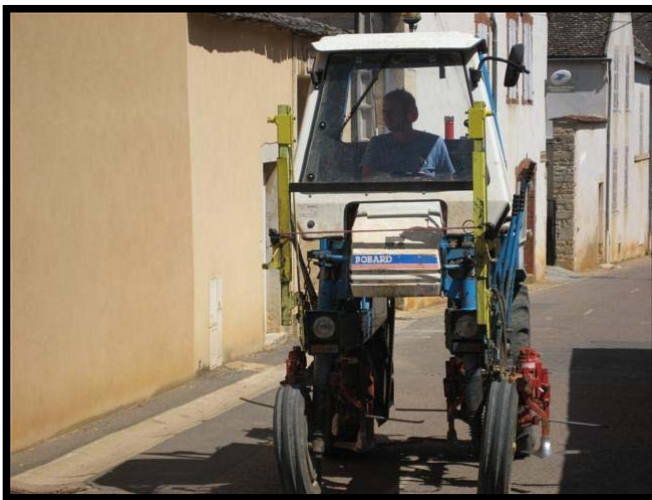
A locally made tractor for narrow row high density viticulture. A common site around wine region villages.
